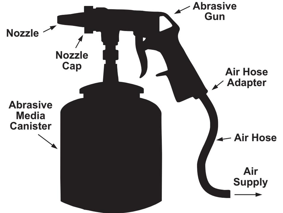
**WARNING:** Never open Abrasive Media Canister when air compressor is attached.
