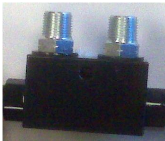
Check valve with BSP-NPT adapters installed
