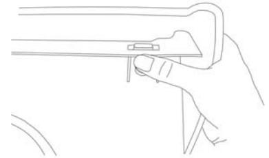
**Step two – attach stair treads:** There should be four adhesive-backed tread covers included with your stairs. Working one step at a time, peel the white paper backing off each tread piece and press firmly into the recessed area on each plastic step. Hold pressure for a few seconds before moving to the next piece. Repeat until all four tread pieces are installed.
