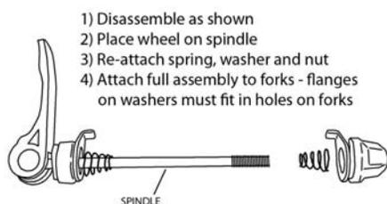
washer and spring from one side (see image). Slide the wheel onto the spindle, then re-assemble the spring, washer and cap nut. Do not tighten the cap nut at this time. Place the wheel in the forks of the gooseneck assembly, so the springs, washers and nuts are all on the outside of the forks. Position the flange on each washer so it engages the hole on each fork, then tighten the cap nut enough so that the cam lever on the opposite side is tight when in the closed position.
