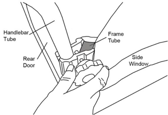
Step 6: Install the cup holder: The large clamp fits over the cushioned section of the handlebar; the small clamp fits over the non-cushioned section. Position the appropriate clamp and attach the cup holder with the nut and screw. Adjust tightness so the cup holder does not “tilt” while in use.
