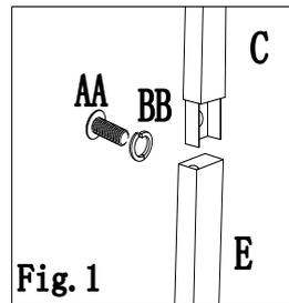
Fig.1: Insert Leg (Upper) (C) into Leg (lower) (E) and secure them with Bolt (AA) and Washer (BB).
