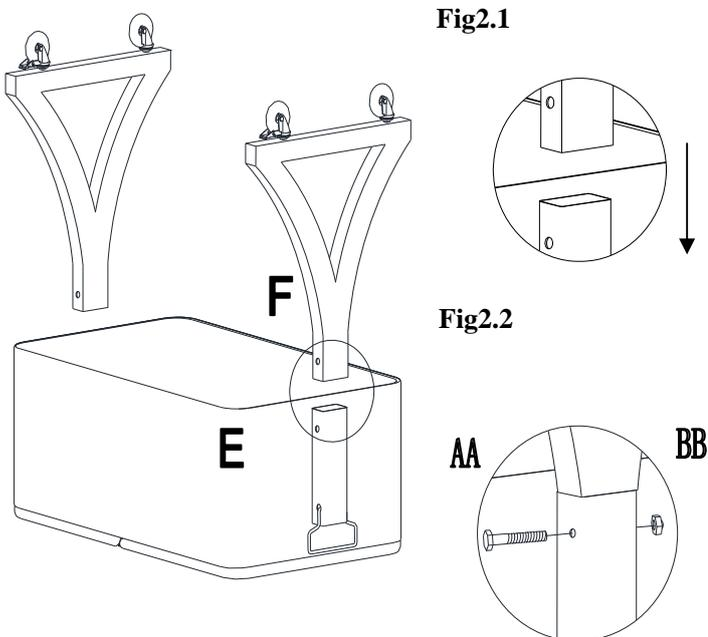
**Step 1:** Install the leg (F) on their relevant position, as pictures by using bolt (AA), nut (BB)
