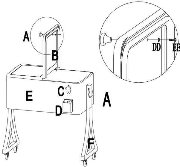
**Step 3:** Connect the knob (A) with lid (B) with bolt(EE) and washer (DD) and tight the bolts.
