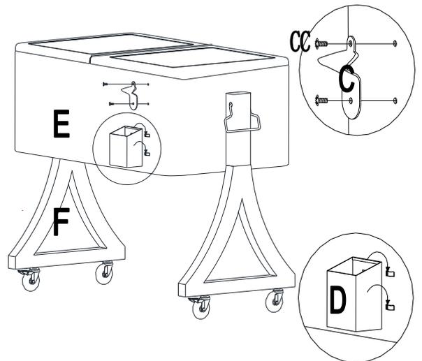
**Step 2:** Connect bottle opener(C) with body (E) with bolt (CC). Stuck the cap catcher (D) into the relevant position.
