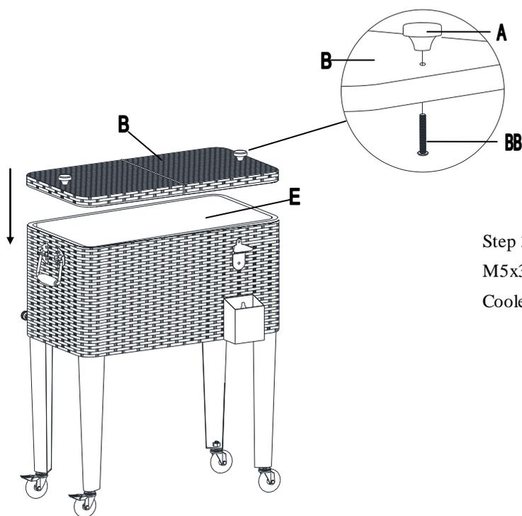
Step 3: Assemble Lids (A) and Lid (B) with Bolt M5x35 (BB). Then place the lid on the frame of the Cooler Body (E).
