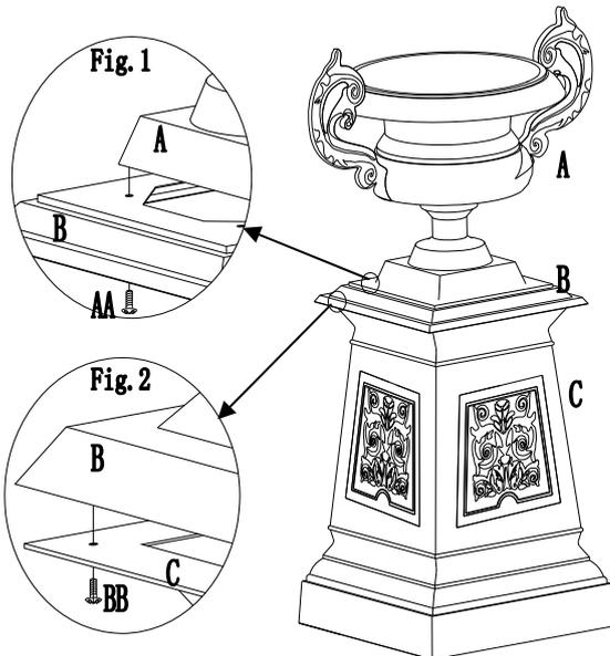
Fig. 2: Place the assembled upper part onto the base (C), then tighten with bolt (BB).
