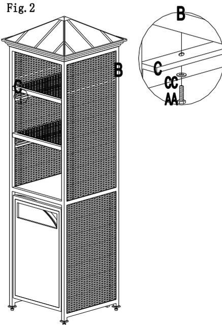
Fig.2: Attach two shelves (C) to frame (B) using 8 pieces M6x20 bolts (AA) and 8 pieces M6 washers (CC).
