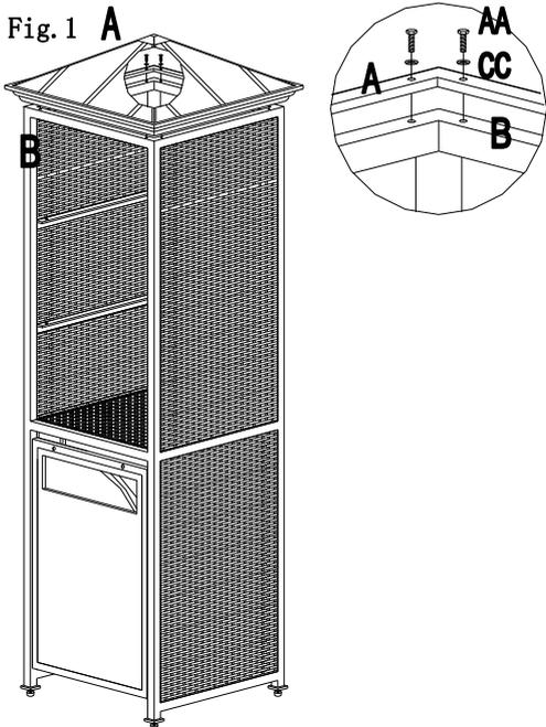
Fig.1: Attach the top (A) to frame (B) using 8 pieces M6x20 bolts (AA) and 8 pieces M6 washers (CC).
