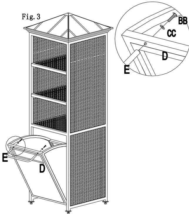
**Fig.3:** Attach the handle (E) to trash can (D) using 2 pieces M6x30 bolts (CC) and 2 pieces M6 washers (CC).
