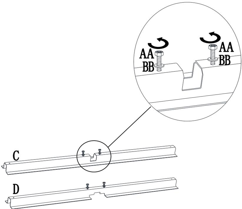
**Step 1:** Take down Bolt (AA) and Washer (BB) (preassembled on Bottom Bar 1 and Bottom Bar 2).
