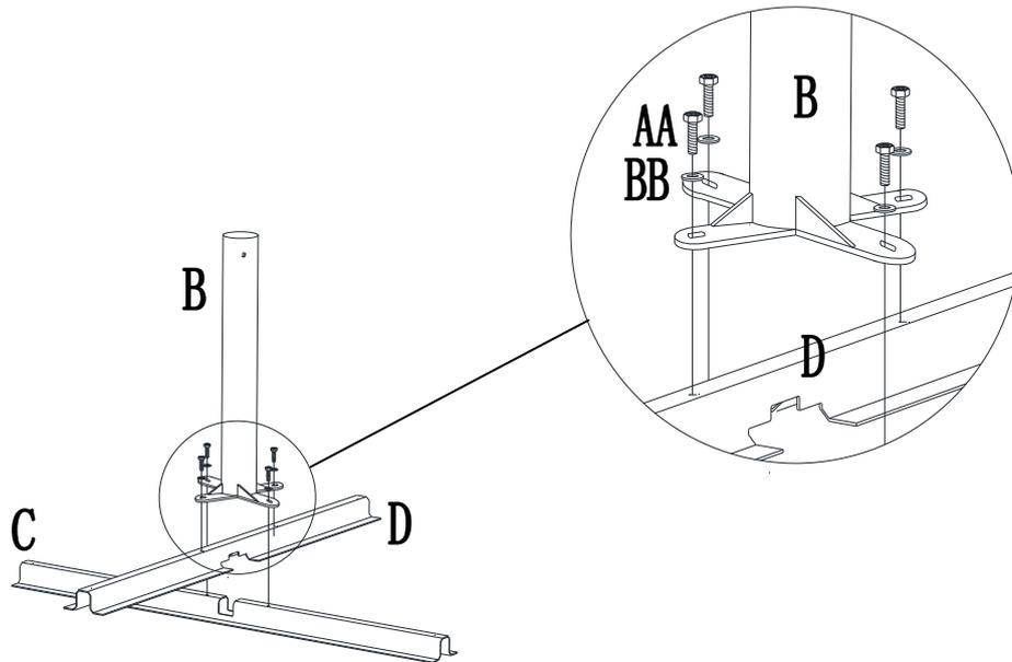
**Step 2:** Cross Bottom Bar 1 (C) and Bottom Bar 2 (D), connect bars with Umbrella Support (B) by Bolt (AA) and Washer (BB).
