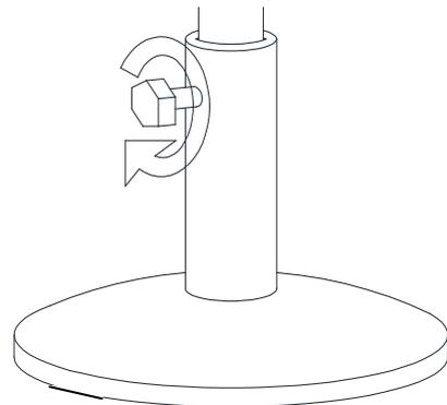
**Step 4:** We recommend that you stand and secure the umbrella to an umbrella base (not included). Secure the umbrella pole firmly by tightening the locking nut.
