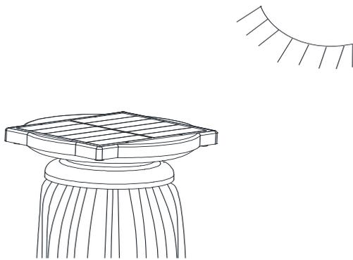
**Step 5:** Put the solar umbrella in the sunlight to charge the batteries before the first use. Make sure to charge the batteries for at least 8 hours before the first use. Otherwise it will shorten lifespan of the batteries and decrease performance. If charging the solar panel while attached to the umbrella, make sure the switch on the pole is in the off position.
