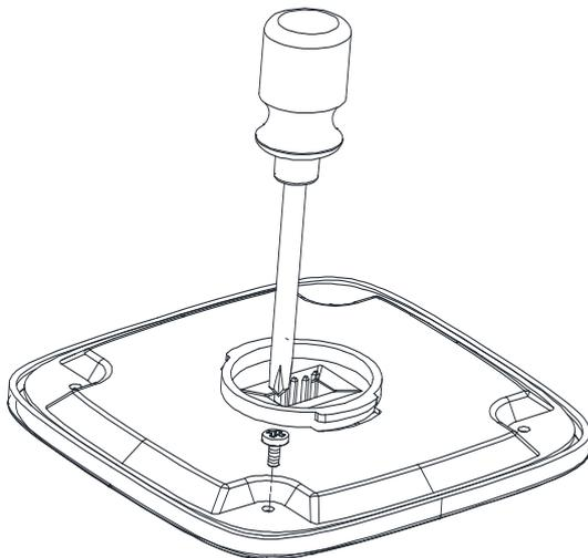
**Step 3:** Put the solar panel upside down on a flat, non-abrasive surface to avoid scratching. Loosen all four (4) screws on the solar panel bottom case.
