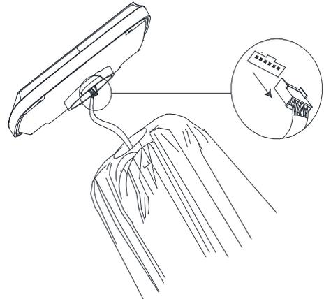
**Step 2:** Pull the plug out of the socket under the solar panel. Pull by holding the plug, not by pulling on the wires.
