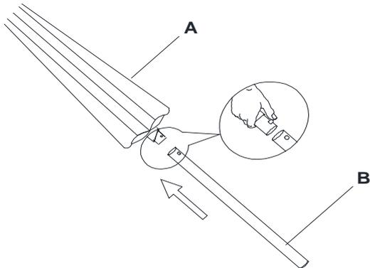
**Step 3:** To assemble the two pole pieces together: Insert the bottom pole into the upper pole while pressing the snap button on the bottom pole until the snap button locks into position.
