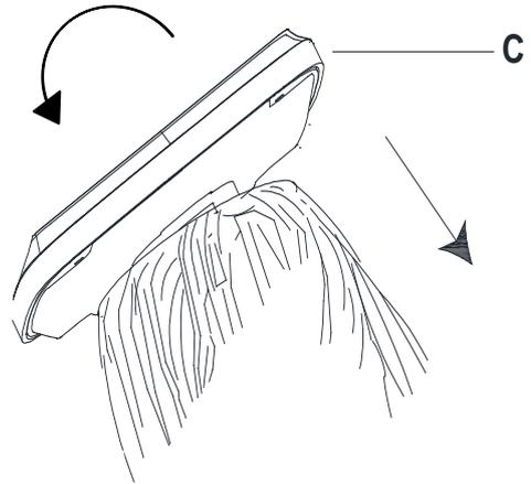
**Step 2:** Put the solar panel on the top of umbrella and hide the plug and wire inside the groove at the top of umbrella. Then turn the solar panel clockwise. Do not over tighten. Please remove the plastic film on the solar panel. \*This protective plastic film is to prevent damage during shipment.
