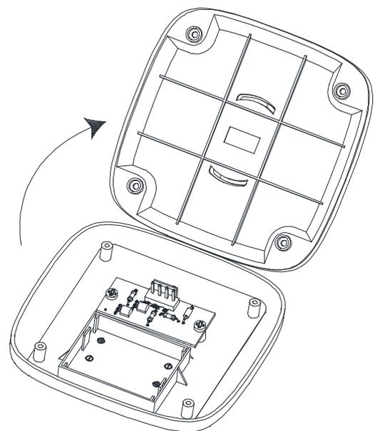
**Step 4:** Carefully open the bottom case and set aside. Fig.10. Replace the batteries, matching the +/- on the batteries with the +/- on the battery case.
