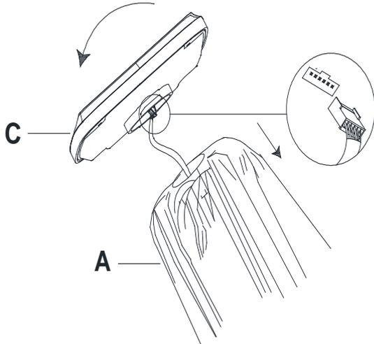
**Step 1:** Insert the plug into the socket under the solar panel(C).
