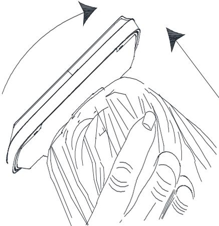
**Step 1:** Twist counterclockwise and remove the solar panel from the top of the umbrella.
