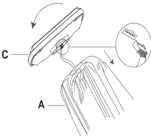
**Step 1:** Find the plug at the top of the Umbrella Shade (A). Insert the plug into the socket under the Solar Panel (C).
