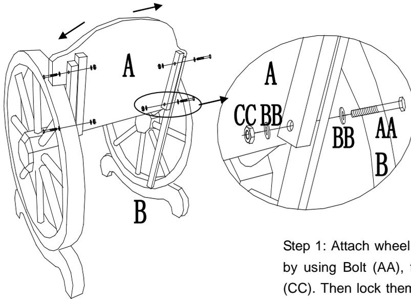
Step 1: Attach wheel support (B) and back (A) by using Bolt (AA), flat washer (BB) and nut (CC). Then lock them tightly as showed in the picture.
