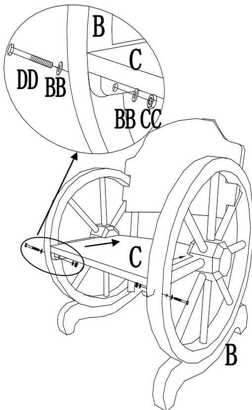
Step 2: Insert seat (C) into the wheel support (B) then fix by bolt (DD), flat washer (BB) and nut (CC).
