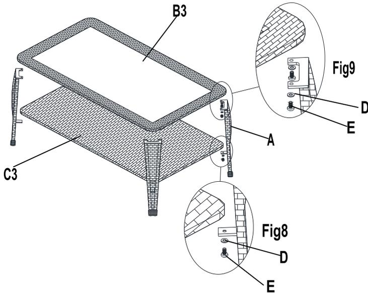
**Fig 8:** Attach table legs (A) to table base (C3) using bolt (E) and flat washer (D), do not tighten at this moment.
