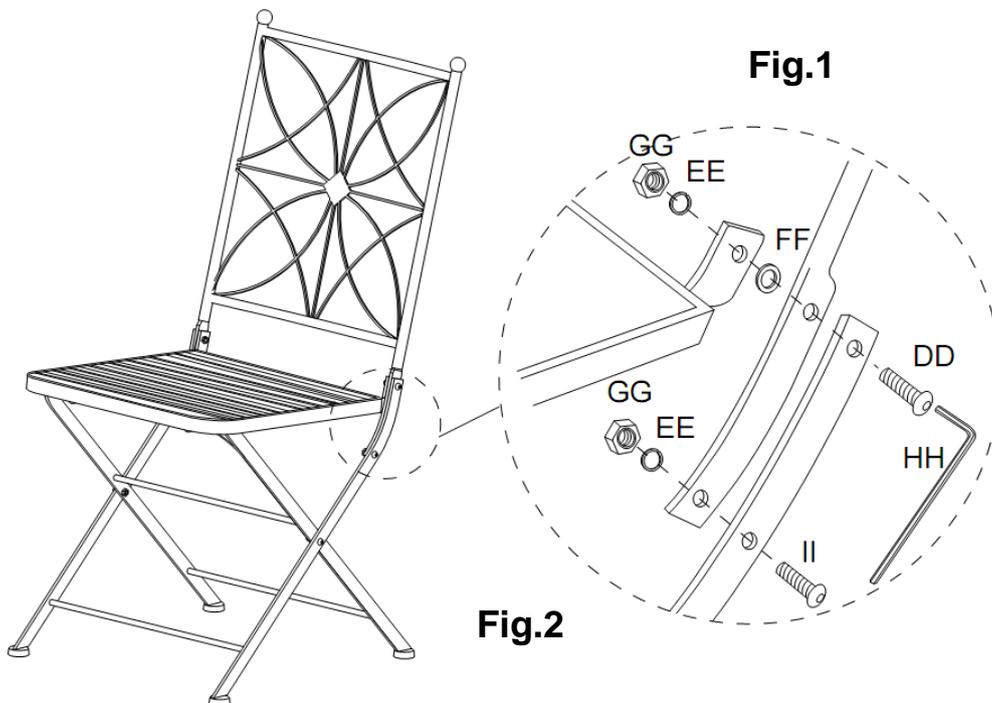
**Fig.1:** Connect Chair Back (A) and Seat (B) with Screw (DD), Flat Washer (FF), Spring Washer (EE), Nut (GG), Wrench (HH), and Wrench (CC), but do not tighten at this step.
