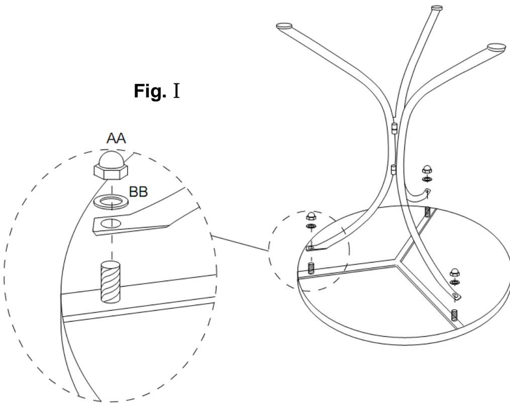
**Fig. I** : Put the Table Top (A) upside down, place the screw hole of Leg (B) onto the screw of Table Top (A), and tighten with Flat Washer (BB) and Nut (AA) by using Wrench (CC). Repeat with the other 2 legs. Then place it upright.
