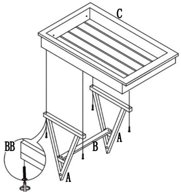
**Step 2:** Attach Triangle side panel (A) and Basket (C) with Bolt (BB).
