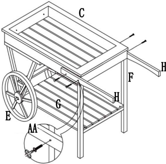
**Step 7:** Attach Armrest batten (H), Basket (C) and Support panel (F) with Bolt (AA).
