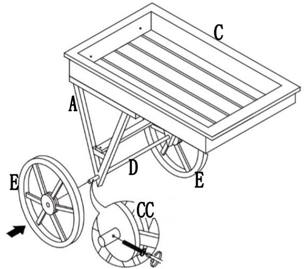
**Step 4:** Attach Wheel (E) and Support bar (D) with Bolt (CC).
