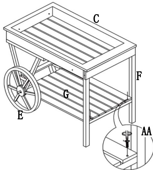
**Step 6:** Attach Shelf (G) and Support panel (F) with Bolt (AA).
