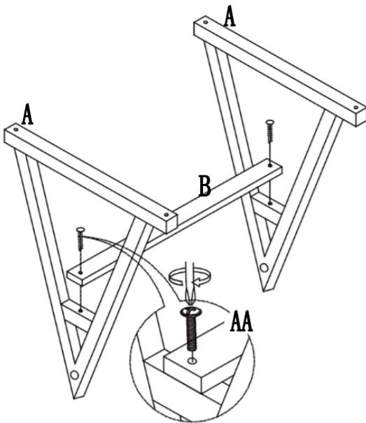
**Step 1:** Attach Triangle side panel (A) and Connect batten (B) with Bolt (AA).
