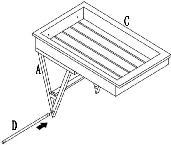
**Step 3:** Insert Support bar (D) into Triangle side panel (A).
