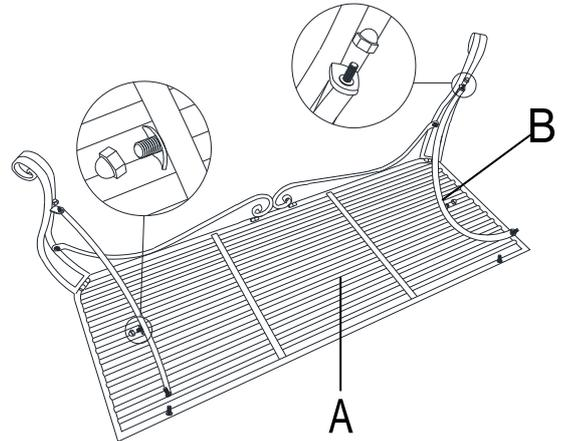
**Step2:** Connect Support tube (B) with Seat (A) by Nut (AA).
