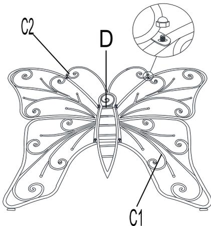
**Step3:** Connect Wings (C1&C2) with Body (D) by Nut (BB).
