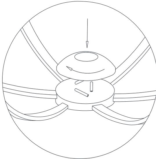
**Step:** Open Cover of battery, put into 3pcs “AA” Battery, and put back cover.
