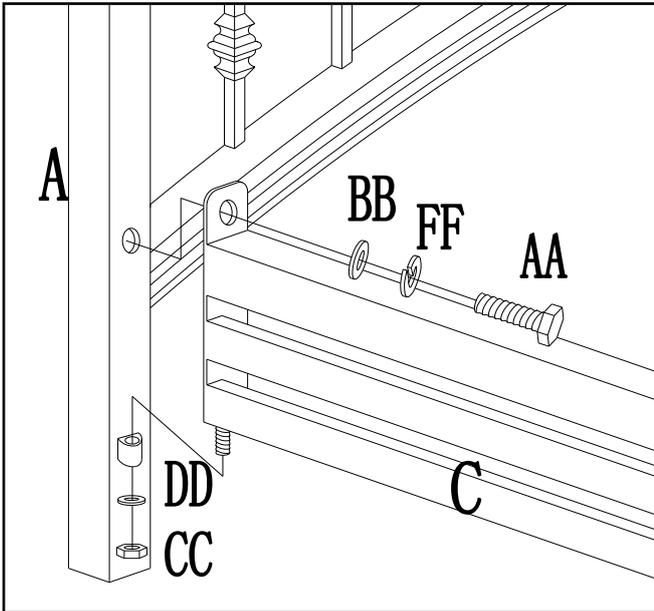
Fig.2: Attach side panel (C) onto bridge railings (A), then lock the lower part of side panel (C) with flat washer (CC) and nut (DD), then lock side panel (C) onto bridge railings (A) with bolt (AA), spring washer (FF) and flat washer (BB), but do not tighten them at this step.
