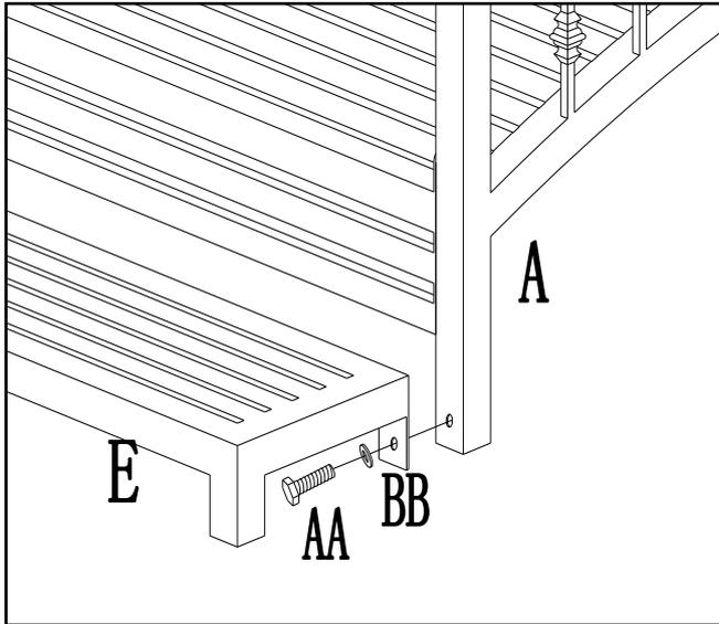
Fig.4: Lock step (E) onto bridge railings (A) with bolt (AA) and flat washer (BB), then tighten all the bolts and nuts with wrench.
