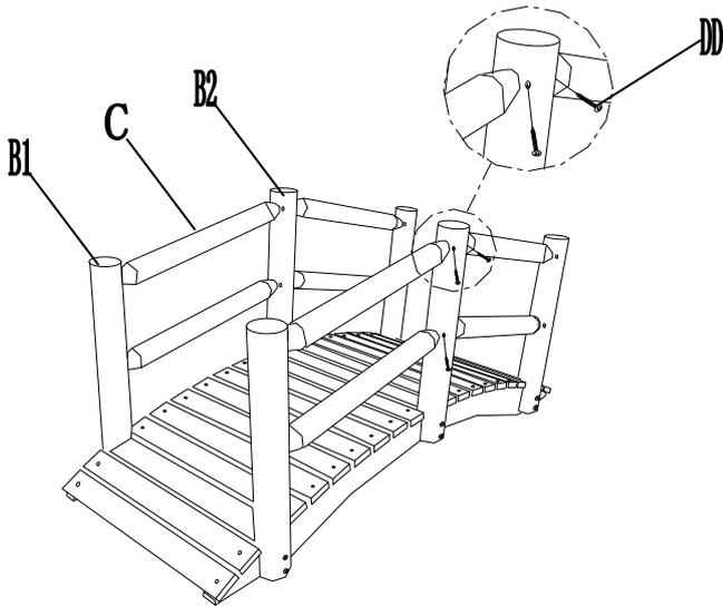
**Step 3:** Adjust left and right column in symmetry, then fasten Guard Bar (C) to Front & Back Column (B1) and Middle Column (B2) with Screw (DD) respectively.
