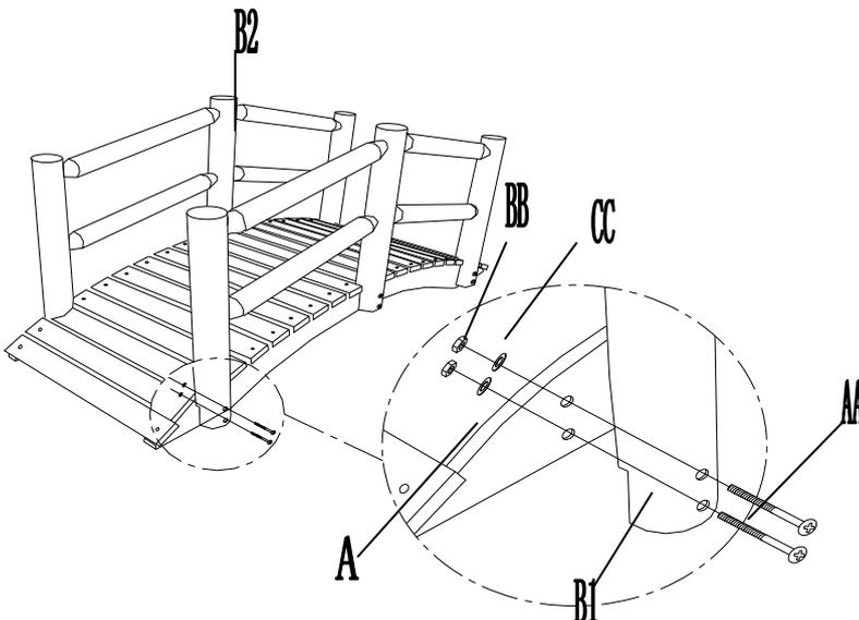
**Step 2:** Attach Front & Back Column (B1) to Bridge Body (A) with Bolt AA, Washer CC, and Nut BB. Repeat this step for Middle Column (B2).
