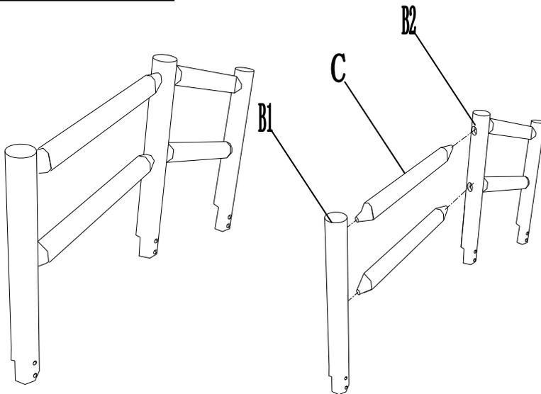
**Step 1:** Insert Guard Bar(C) into Front & Back Column (B1) and Middle Column (B2). (Do not use Screw now.)
