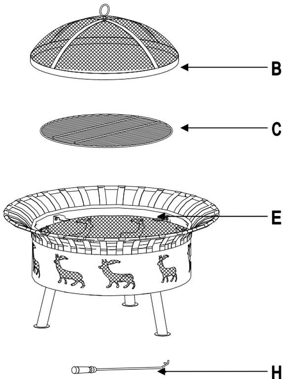
**Step 5:** Turn around the fire pit to have it stand upright in normal status. Put Grate (C) and Screen (B) onto the Grill Supporter (E). Then place Poker (H) is beside of fire pit.
