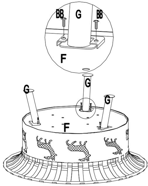
**Step 4:** Reverse Fire bowl (F) and place it on the level ground, insert the square end of Leg (G) into the slot of Fire bowl (F), use Bolts (BB) to secure it. Do the same for the other two legs. (Please use the Screwdriver to tighten).
