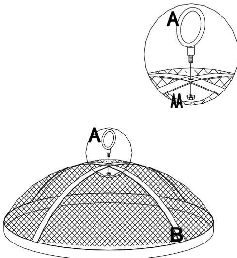
**Step 1:** Connect Lift handle (A) with Screen (B) and use Flange Nuts (AA) to fix them.
