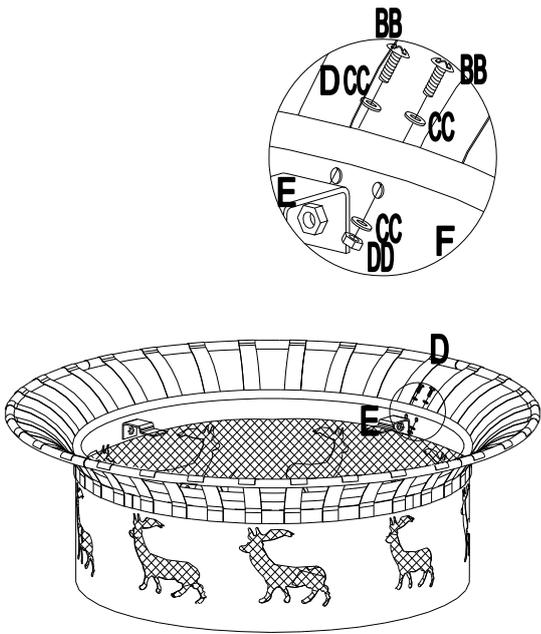
**Step 3:** Connect the Grill supporter (E) and Decorative Rail (D) with 4pcs Bolts (BB), Washer (CC), then to connect fire bowl (F) and Decorative Rail (D) with 4pcs Bolts 4pcs Nuts (M) and 8pcs Washer (CC).
