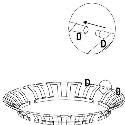
**Step 2:** Put 4pcs Decorative Rail (D) as photo. Then join the Decorative rails (D) together one by one, final to be cycle.
