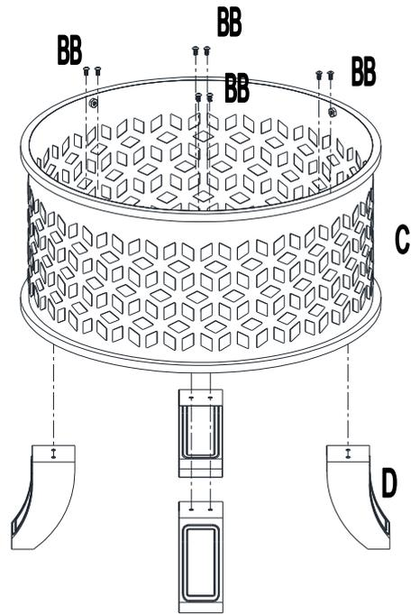
**Step 2:** Connect Fire Bowl (C) with Leg (D) by 8 Screw (BB).
