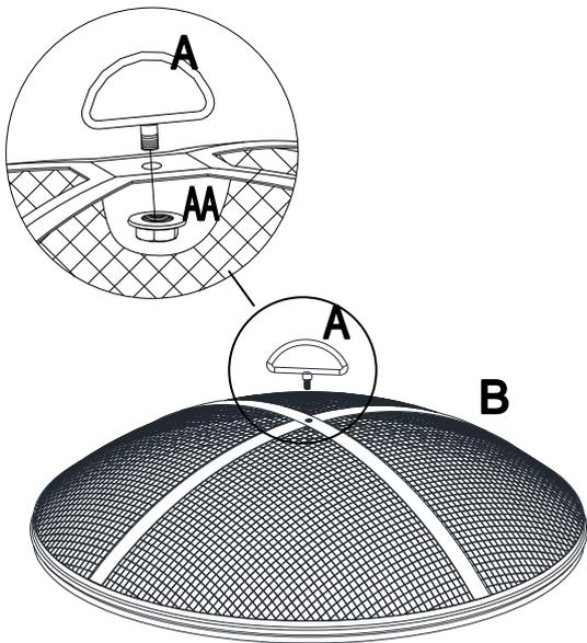
**Step 1:** Attach Handle (A) to Screen (B) with Nut (AA).
