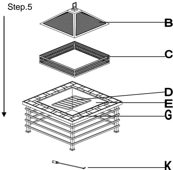
5. Turn the assembled top and put bowl into top (G). Then add the fire grate (D), screen (C) and screen (B) orderly. Put the poker (H) aside ready to use.
