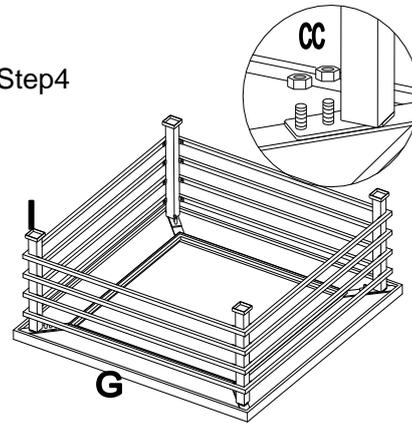
4. Turn the assembled frame upside down on the back of the top (G), and connect them by using 8 nut (CC). Then tighten all screw by using wrench (DD).
