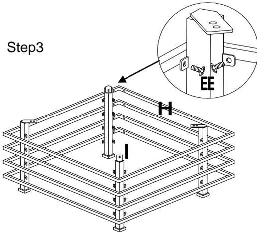
3. Connect leg (I) and Connect ring (H) by using 32 crews (EE), but not tighten.
