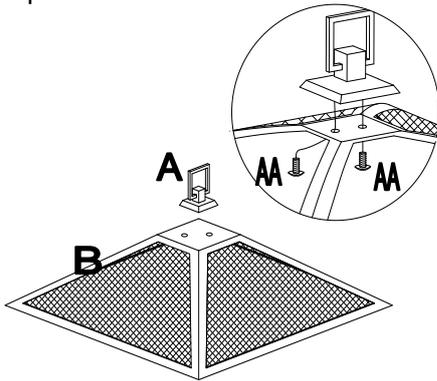
1. Connect handle (A) and screen (B) by using two screws (AA).
