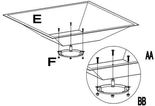
2. Connect bowl (E) and ashtray (F) by using three screws (AA) and three nut (BB).
