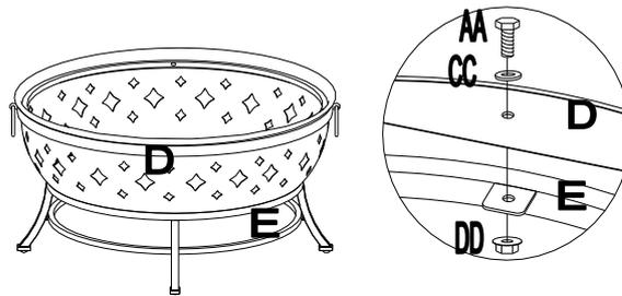
4. Turn over the bowl (D) and contact it with Upper ring (E) by Bolt (AA), Flat washer (CC), Nut (DD) and tighten them with Wrench (EE). (the bowl above needs to be shown upside down.)
