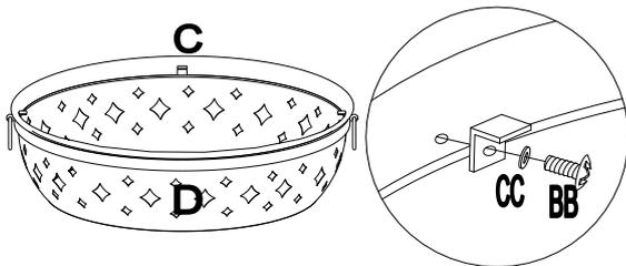
3. Connect Support support (C) and Bowl (D) with bolt (BB) and Flat washer (CC).
