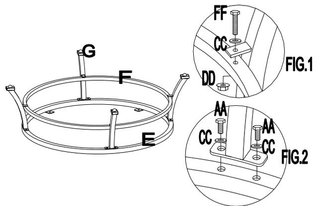
2. Attach Leg (G) to Bottom ring (F) by using Bolt (FF), Flat washer (CC), and Nut (DD). Do not tighten them at this step. Next, attach Leg (G) to Upper ring (E) by using Bolt (AA) and Flat washer (CC). Tighten all bolts with Wrench (EE).
