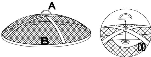
1. Connect Screen handle (A) and Mesh Screen (B) by using Nut (DD). Use Wrench (EE).
