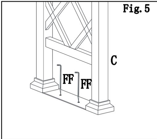
**Step 5:** Secure the assembled arbor to ground with stakes (FF).
