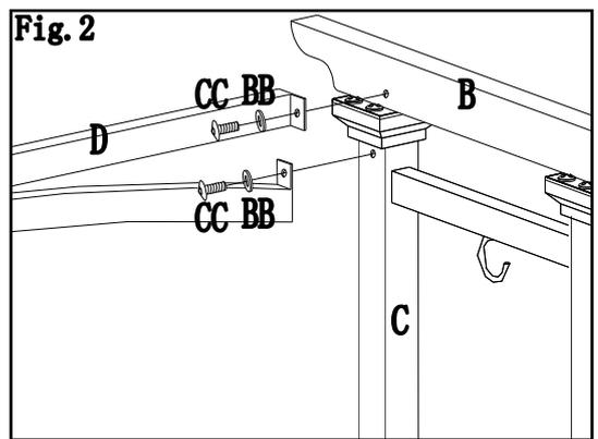
**Step 2:** Attach screen supporting bar (D) to screen (C) and supporting bar (B) with hex bolts (CC) and washers (BB).
