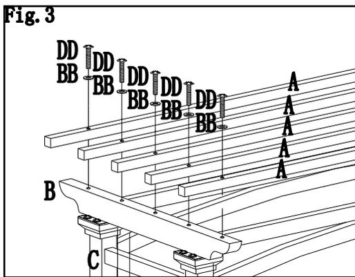
**Step 3:** Attach beam (A) to supporting bar (B) with bolts (DD) and washers (BB).
