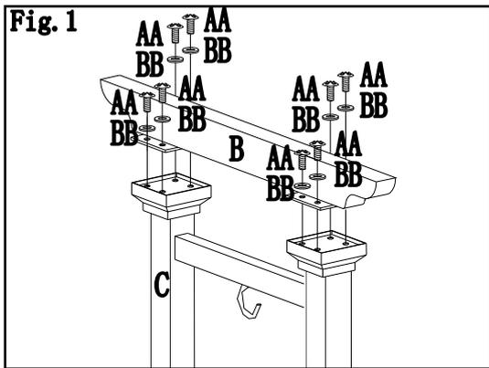
**Step 1:** Attach supporting bar (B) to screen (C) with bolts (AA) and washers (BB).
