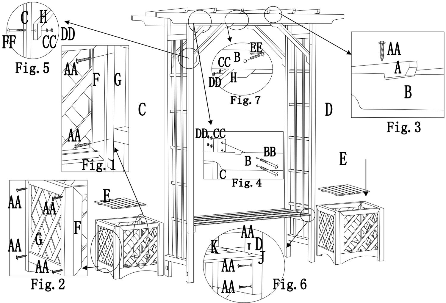
**Fig.1:** Connect Flowerpot Front/Rear Plate (F) to Flowerpot Side Plate (G) using Self-taping Screw (AA).
