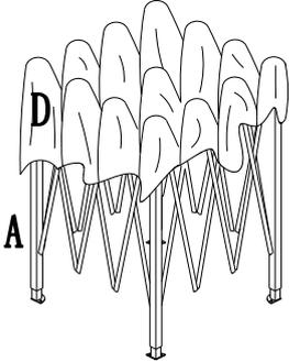
Step 2: Place the gazebo frame (A) upright and attach the large canopy (D) on top. Have four people holding the corner posts and pulling outwards.
