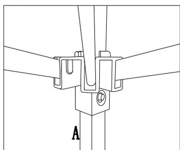
Step 5: Pull the plastic buckle of the gazebo (A) post to the spring buckle and secure it.
