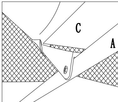
Step 3: Attach the Small canopy (C) to the plastic parts of the small top when pulling the gazebo outwards.
