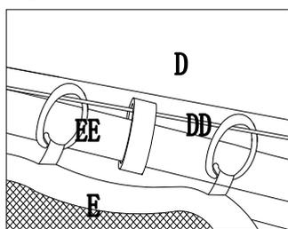
Step 8: Pass the netting rope (DD) through the loop on the large canopy (D) and tighten netting rope (DD) in place. Attach mosquito netting (E) to the netting rope by using rings (EE).
