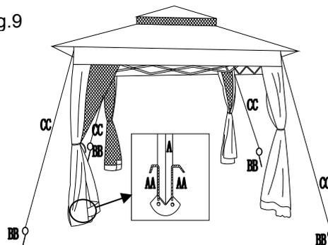
Step 9: Secure the gazebo to the ground by using stakes (AA) and ropes (CC); tighten ropes on the corners of the large canopy (D) and secure each rope with large stakes (BB).
