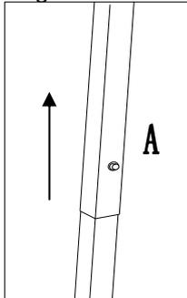
Step 6: Pull the gazebo post upwards to the spring buckle to secure in place.
