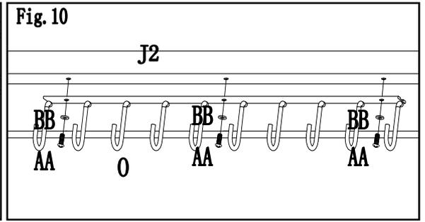
**Fig.10:** Attach hook rack (O) to glass side bar J2 by using bolt (AA) and flat washer (BB).
