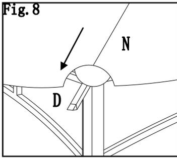
**Fig.8:** Spread the large canopy (N), put large canopy onto assembled beam (D), then cover four corners
