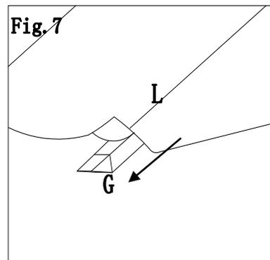
**Fig.7:** Spread the small canopy (L), Put small canopy onto assembled small top pole, then cover four corners.
