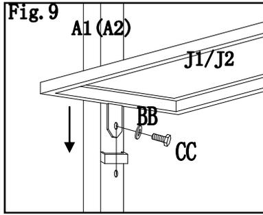
**Fig.9:** Attach the connector of glass side bar J1 (J2) to U shaped plate on the post then tighten the connections by bolt (CC) and flat washer (BB)
