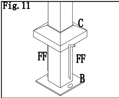
**Fig.11:** Lift up the base cover(C), secure the completely assembled gazebo into the ground by using “7” stakes (FF).
