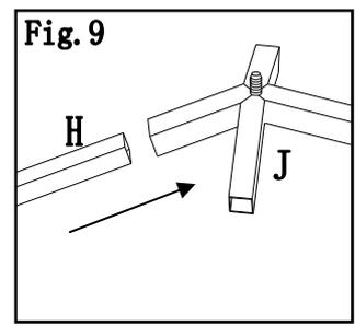
**Fig.9:** Insert pole (H) into center connector (J)
