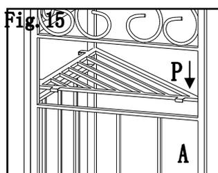
**Fig.15:** Install shelf (P) at the middle distance of screen (A)
