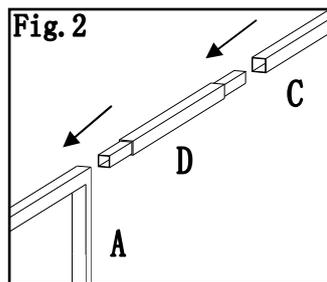
**Fig.2:** Combine long side support pole 1(C) with long side support pole 2(D), insert then install long side support pole 2 (D) to screen (A)
