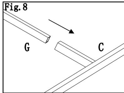
**Fig.8:** Insert pole (G) into long side support pole1(C),insert pole(F) with the same way, Then slip over the big canopy(Q) on the big top, do not fully spread.
