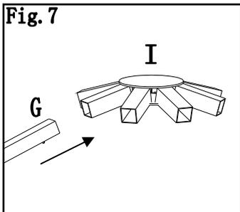
**Fig.7:** Insert pole (G) into center connector (I)
