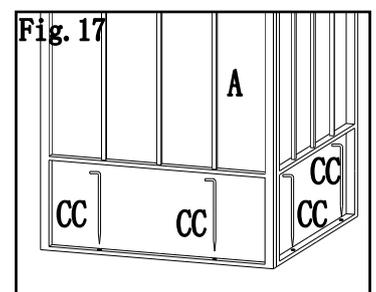
**Fig.17:** Fix the completely assembled gazebo by stake (CC)
