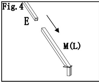
**Fig.4:** Insert pole (E) into corner connector (M,L)
