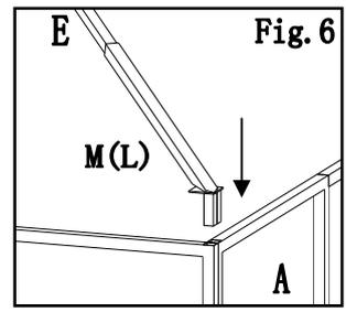
**Fig.6:** Insert installed corner connector (M, L), into screen (A)
