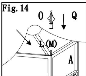
**Fig.14:** Slip over the big canopy (Q) on four corners of screen (A), install corner finial (O) on the pole as picture
