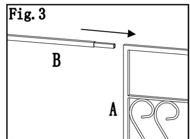
**Fig.3:** Install short side support pole (B) to screen (A)
