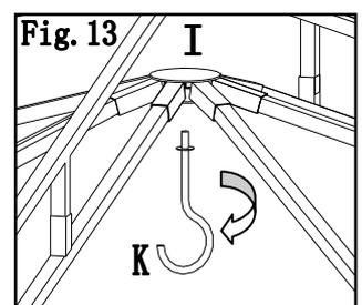
**Fig.13:** Attach the top hook (K) to center connector (I)
