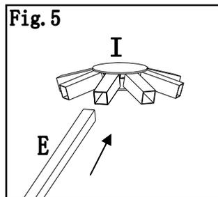
**Fig.5:** Insert pole (E) into center connector (I)
