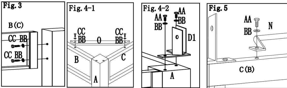
Fig.3: Attach the Long horizontal screen (B) and Short horizontal screen (C) to the Post (A) by using Bolt (CC) and Washer (BB).
