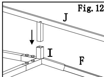
Fig.12: Lay the Big canopy (R) and then Middle canopy(Q) on the top, and do not spread them at this time ,then attach the assembled small top to the big top connector (I) by putting the tube of the slanting bar(J) into the tube of the big top connector (I).
