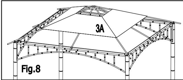
**Fig.8:** Put Canopy for the second roof (3A) onto top roof. Do not complete it here in order to assemble the second roof.
