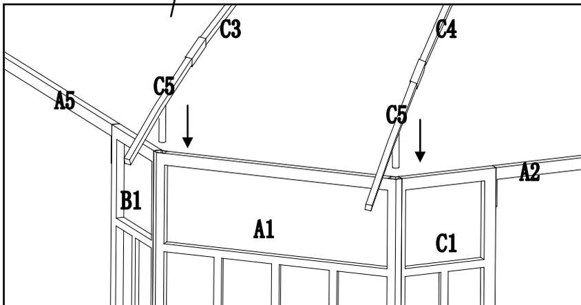
Step7: Insert arch bar connector (C5) into big screen (A1).
