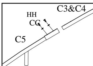
Step5: Insert arch bar 1(C3) and arch bar 2 (C4) into Arch bar connector (C5), fully tighten with bolt (HH) and flat washer (CC).
