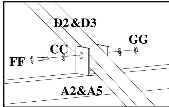
Step9: Connect Side Supporting Bar (D3&D2) and bar (A2&A5) with bolt (FF), washer (CC) and nut (GG).
