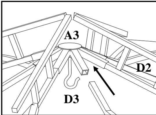
Step8: Insert side supporting bar-Short (D2) and side supporting bar-Long (D3) into larger roof connector (A3).
