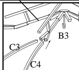
Step6: Insert arch bar 1(C3) and arch bar 2 (C4) into top roof supporter (B3).
