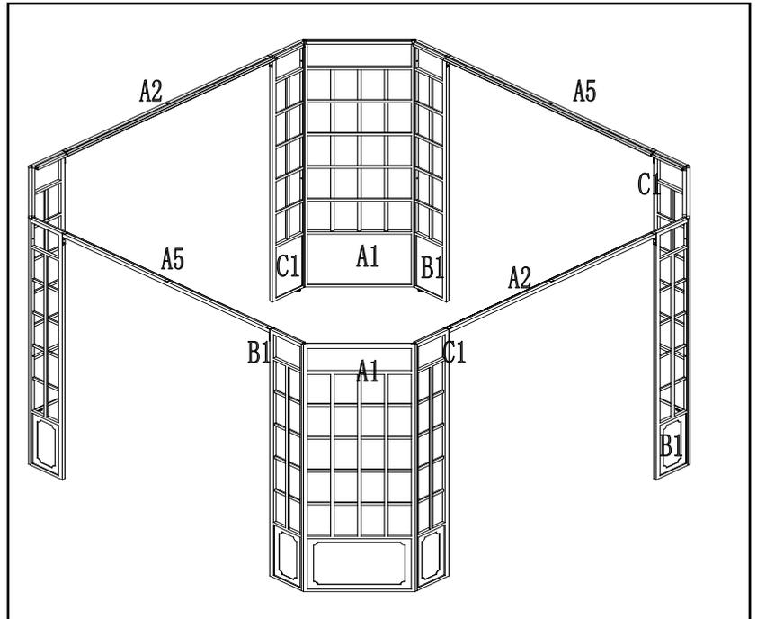
Step2: Connect long bar (A2) and left screen (B1), long bar (A2) and right screen (C1) with bolt (BB) and washer (CC). Connect short bar (A5) and left screen (B1), short bar (A5) and right screen (C1) in the same way.
