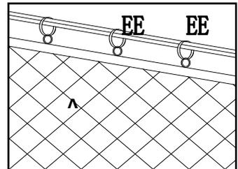
Step11: Attach Mosquito netting (A4) onto bar (A2, A5) with Plastic ring (EE).
