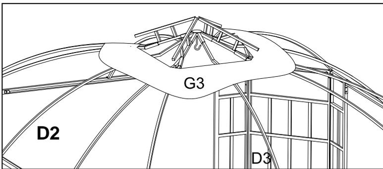
Step10: Put Larger Canopy (G3) on to the top frame. Do not unfold it completely at this time.
