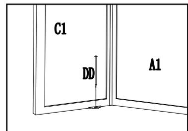
Step12: Secure the completely assembled gazebo by stake (DD).
