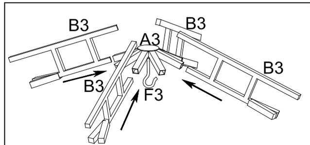
Step4: Insert top roof supporter (B3) into larger roof connector (A3).
