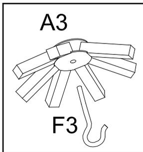
Step3: Attach center hook (F3) to larger roof connector (A3).
