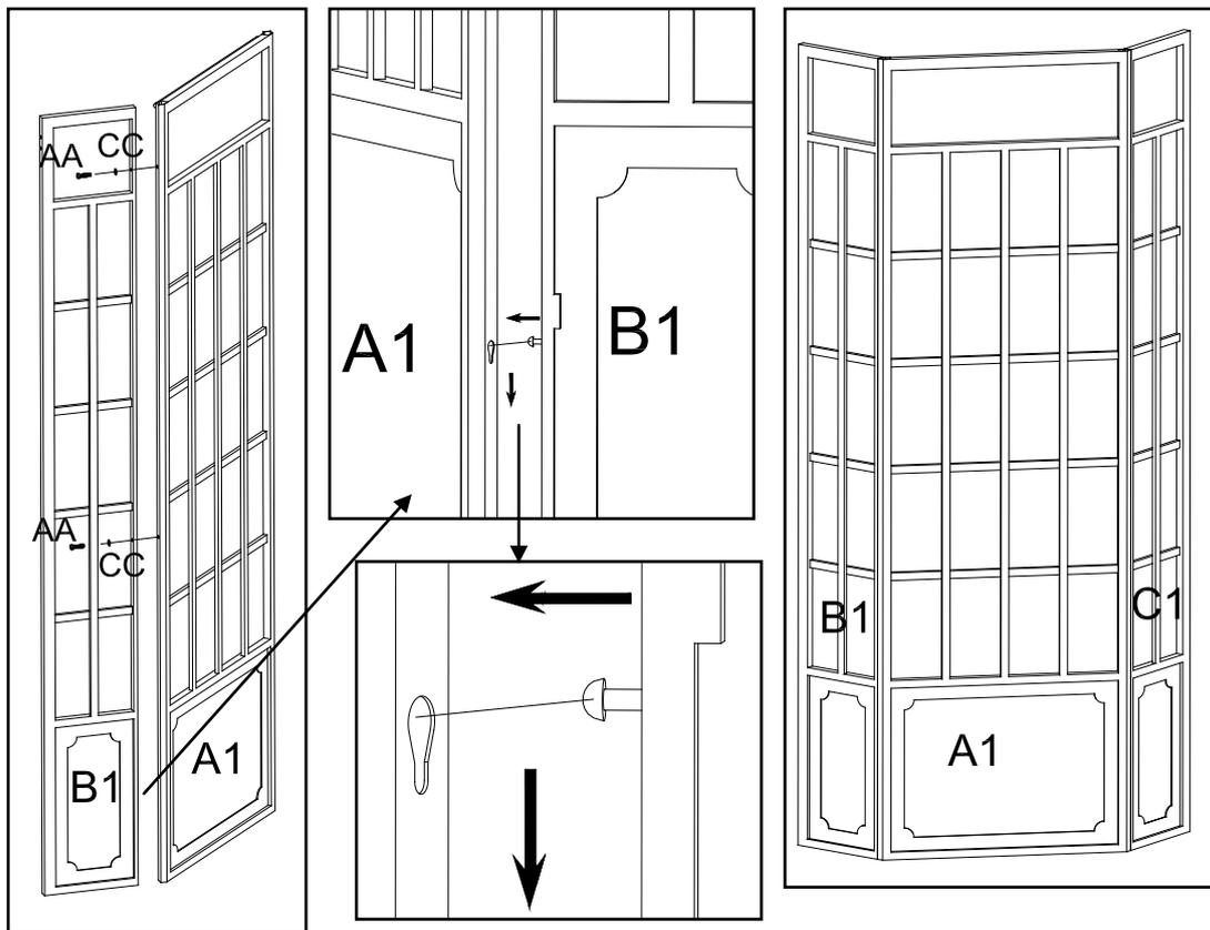
Step1: Insert the left screen (B1) into the big screen (A1), pull it down to attach them, then use screw (AA), washer (CC) to secure left screen (B1) and big screen (A1). Do the same for right screen (C1) and big screen (A1).
