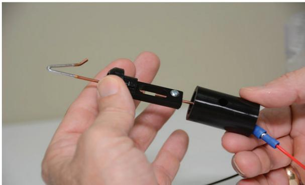
4. To re-assemble place the lower portion of the Knocker back into position and rotate clockwise to lock into position.
