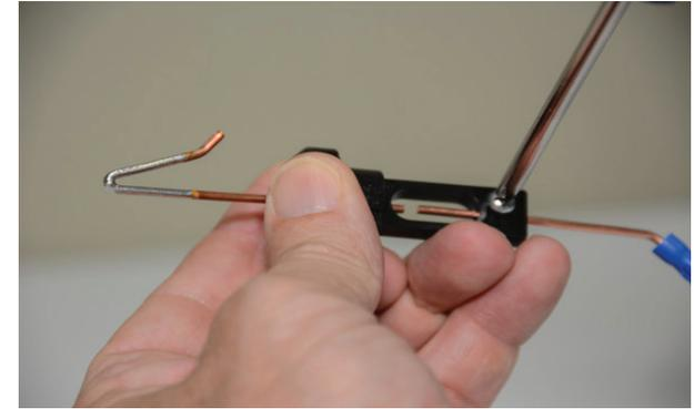
2. Loosen the small screw just enough so you can move the bottom electrode at the end of the red wire in and out.
