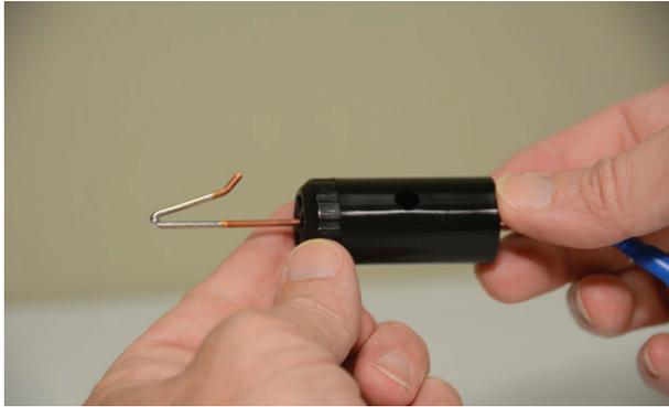
1. Hold the Knocker with both hands and rotate the lower portion of the Knocker counter clock wise and slide the knocker down and out of your way.
