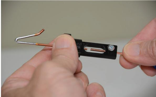
3. With the fence box on adjust the Spark Gap between the Electrodes, wider until it stops arcing. Then keep readjusting the gap smaller until the light begins to flash with every pulse of the Fence Charger. Then tighten screw.
