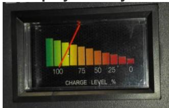
The ammeter indicates the battery capacity by the percentage of battery capacity.
