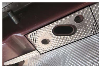
Trim heat shield in area shown – Drivers side
