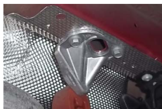
Remove exhaust hanger – Drivers side
