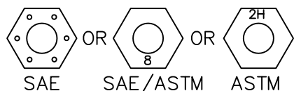
HEAD MARKING OF GR8 BOLT
