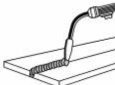
HORIZONTAL POSITION Is performed very much the same as the flat weld except that angle B (see HOLDING THE TORCH) is such that the wire, directed more toward the metal above the weld joint is to help
