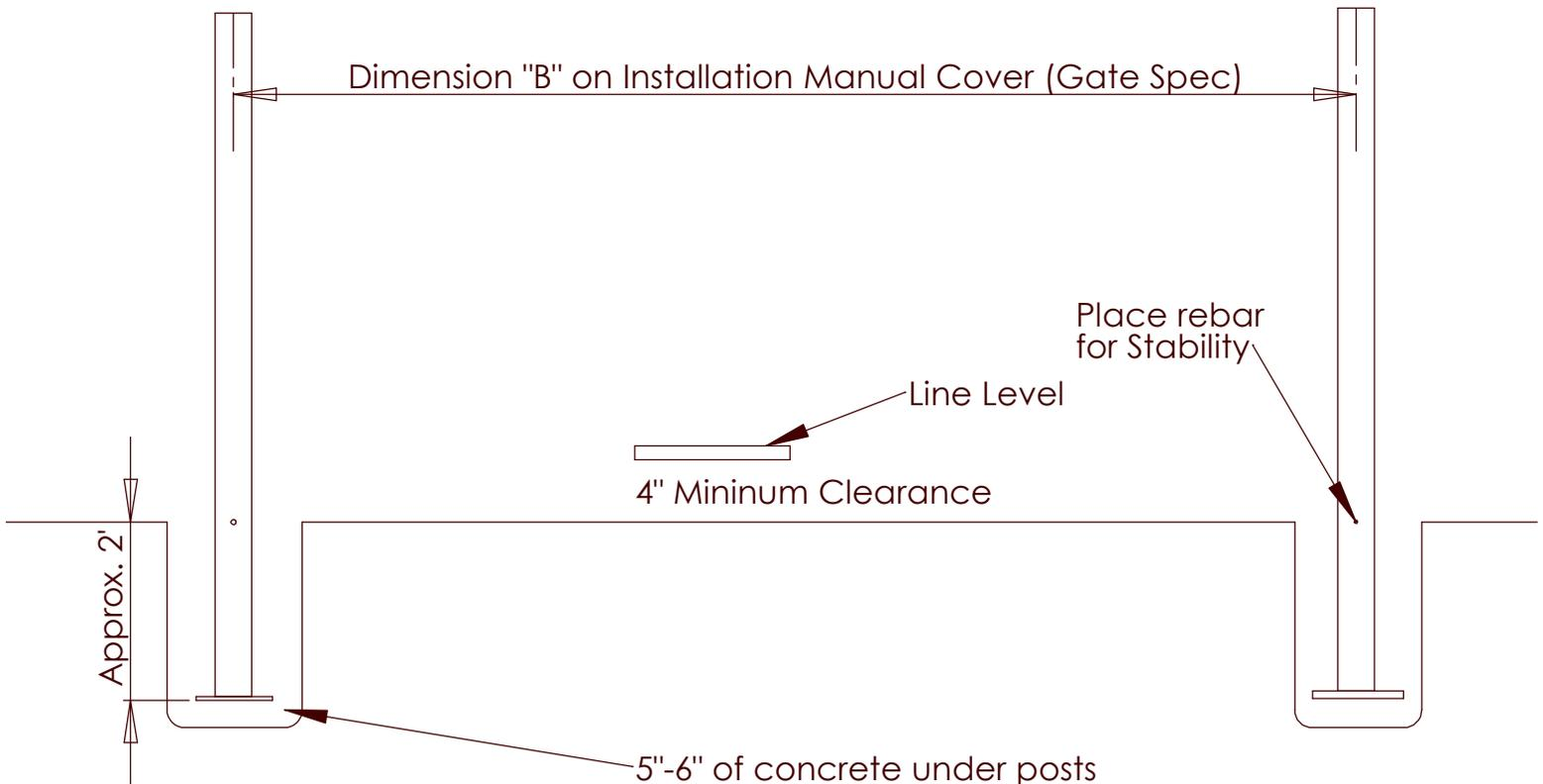
If ground is not level shim rebar with wooden wedges and blocks supplied to level across drive.
