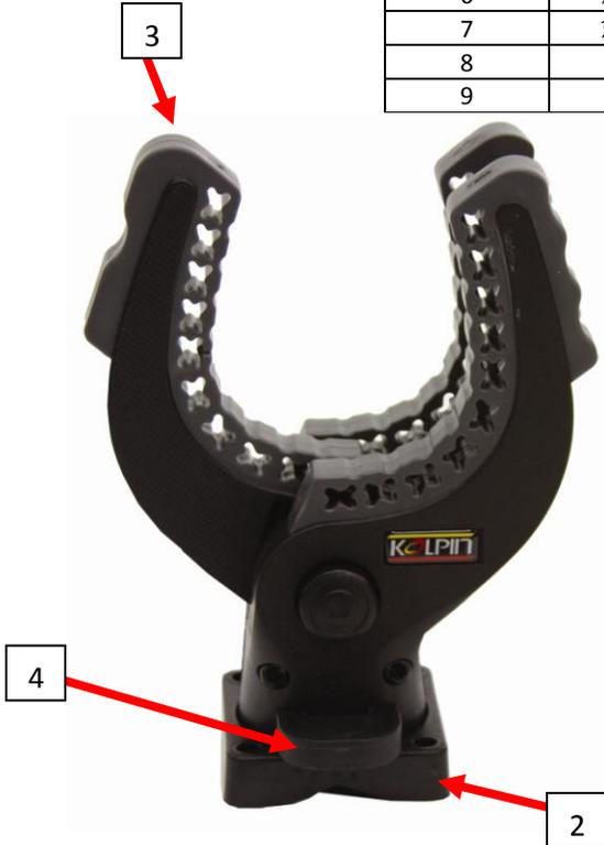
These grips are designed to quickly and easily mount to the Roll Cage of a UTV or Rack of an ATV. They fit tubing sizes from Ø5/8" to Ø2.00". Note: Hardware provided is based on the biggest tube diameter. You may need to trim the excess threads once installed. Failure to do so may result damage to your machine. Note: The grip can be used in the vertical and horizontal positions.
