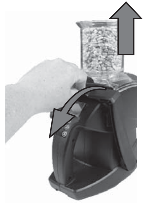
Figure 3. Pull level arm forward. Lift hopper up.
