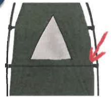
ATTACH ONE SPREADER ROD TO EACH END OF TENT (1/2 WAY DOWN)
