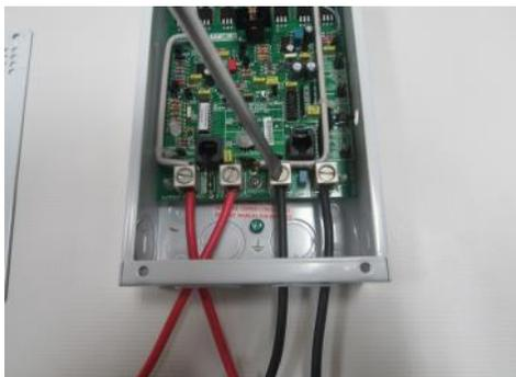
**Step 5:** Attach the lug end of the red cable to the positive terminal on the battery and the bare end to the Battery + input on the charge controller. Attach the lug end of the black cable to the negative terminal on the battery and the bare end to the Battery - input on the charge controller.
