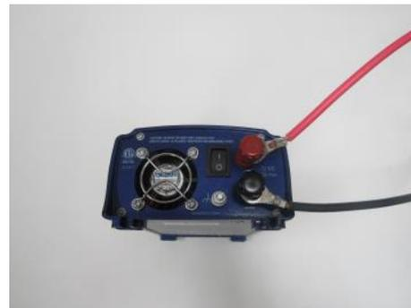
**Step 10:** Uncover the panel. As the day progresses, you should see an increasing number of consecutive green flashes, until the LED is solid green indicating that the charge controller is in float mode. At this point the battery can be used to provide power (turn the inverter on and plug your AC devices into it for power).
