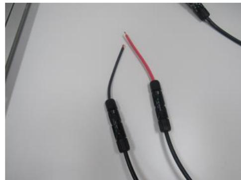
**Step 9:** Connect the red (positive) and black (negative) 5-foot cable from battery to inverter.
