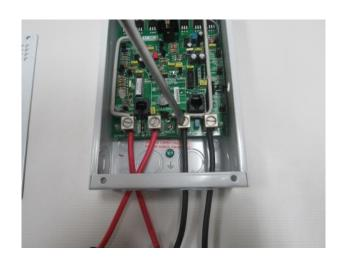
**Step 8:** Uncover the panel. As the day progresses, you should see an increasing number of consecutive green flashes, until the LED is solid green indicating that the charge controller is in "float" mode". At this point the battery can be used to provide power.
