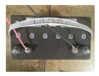
**Step 6:** Connect the MC4 outputs of the panel (or, if you are using MC4 extension cables, the MC4 outputs of those) to the 6" MC4-to-bare wire pair as shown below:
