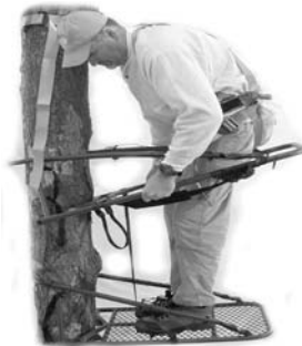
FIGURE 25 LIFT SEATING PLATFORM
