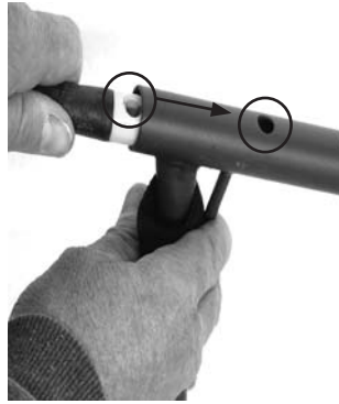
FIGURE 2 INSERT CABLE ASSEMBLY INTO SPREADER ARMS (LINE-UP SPREADER ARM AND CABLE HOLES)
