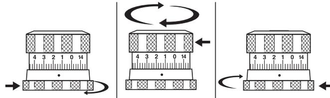
Note: If a large amount of windage and elevation adjustments are needed to bore sight, make half of the scales available adjustments at a time for the windage and elevation.
