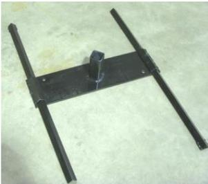
6) Slide the post into the socket in the Static Base. The post is bent to present an angled target face to the bullet strike, in order to direct the fragments downwards.
