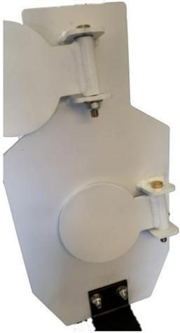
1) Lay target face down on table, insert the grade 8 carriage bolt with the round head on the face that is exposed to bullet strikes. The two Grade 8 carriage bolts, the 4 ½ inch Hex Grade 8 bolt, 3 hardened flat washers and 3 locknuts are shipped with the static stand. Do not use any lower grade bolt, as the head will be damaged by bullet strikes.
