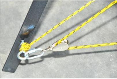
8) Install 5/16-18 eyebolt, loop and pulley to the left rear leg, and on the end of the reset arm. Thread rope from the bottom through the pulley, then up to the end of the reset arm, through that pulley, and then tie end of the rope to the 5/16 eyebolt in the leg.
