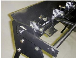
4) Place one large washer on the 1 inch stud on the right end of the assembly, then install the reset arm on the stud, while allowing the reset assembly to rest on the support bars. Do not try to install the other end of the assembly at this time.
