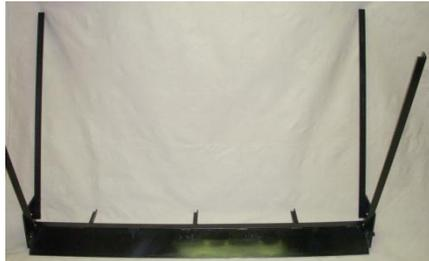
2) Note the flanges are forward, and the nuts are on the inside of the legs. Install the other two legs.
