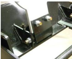
7) Add target to each station, using the grade 8 Carriage bolt, washer and locknut. Targets are on the front of the plate, with bolt heads to the front of the target. Tighten nuts securely.
