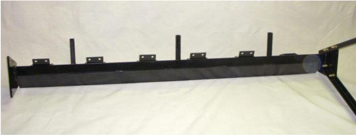
1) Two people are needed for the assembly. Lay main rack assembly on the ground, and install legs on the inside of the end plates, and with the leg flanges on the front side (shooter's side) of the rack. Use the 1/2-13 X 1 1/2 grade 8 hex bolt, lock washer and nut to attach the legs. Insure you mount the leg with the 5/16 inch hole near the bottom at the left rear, when the assembly is viewed from the shooters side.
