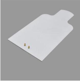
1) Place target on table with end of target with holes off the table, or place on ground with blocks under the end with holes. Assembly is a two man operation. Place the two Grade 8 Carriage bolts in the holes. Never use a lower grade bolt, as they may be damaged by the impacts.
