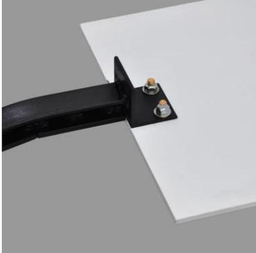
1) Mount the target body to the post with the two grade 8 hardened 1/2-13 Carriage bolts on the front, with the washers and locknuts on the rear. Never use any lower grade bolt, as they will be damaged by the bullet strikes
