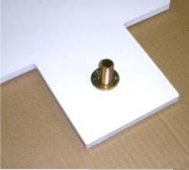
1) Lay target face down on table, insert the grade 8 carriage bolt with the round head on the face that is exposed to bullet strikes. The Grade 8 carriage bolt, two hardened flat washers and a locknut are shipped with the stand. Do not use any lower grade bolt, as the head will be damaged by bullet strikes.
