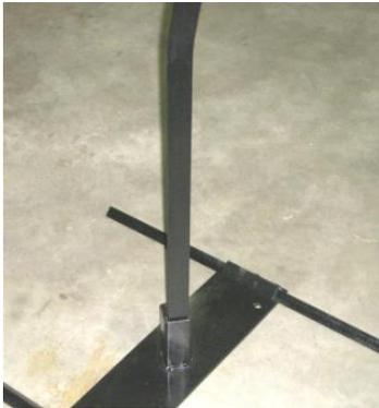
5) Slide the post with target into the socket in the base. The post is bent to present an angled target face to the bullet strike, in order to direct the fragments downwards.
